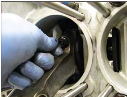
Placing rod half in place and starting top nut.
