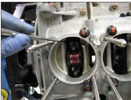
Holding rod end in place with magnet.
