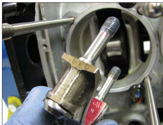
Placing rod end on the crank.
