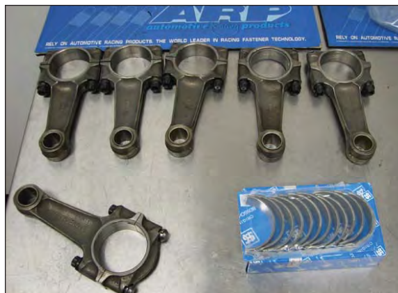
Rods ready for bearings. Normally I will match numbers and halves together with a paint pen so as not to mix up the ends when putting them in the case.
