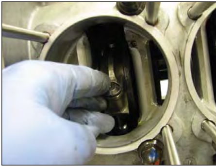
Rotating rod end on crank to face bolts outward.
